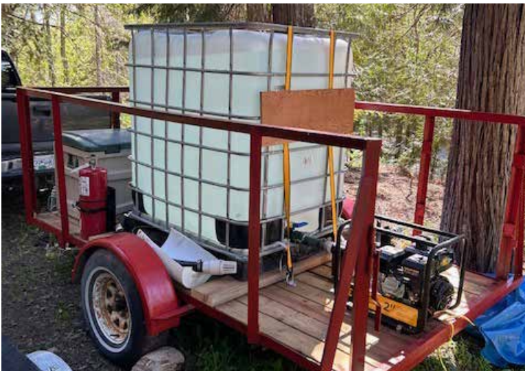
Fire trailer equipped with a 1200 litre tank, 7.5 hp pump, fire hoses and a fire extinguisher.
